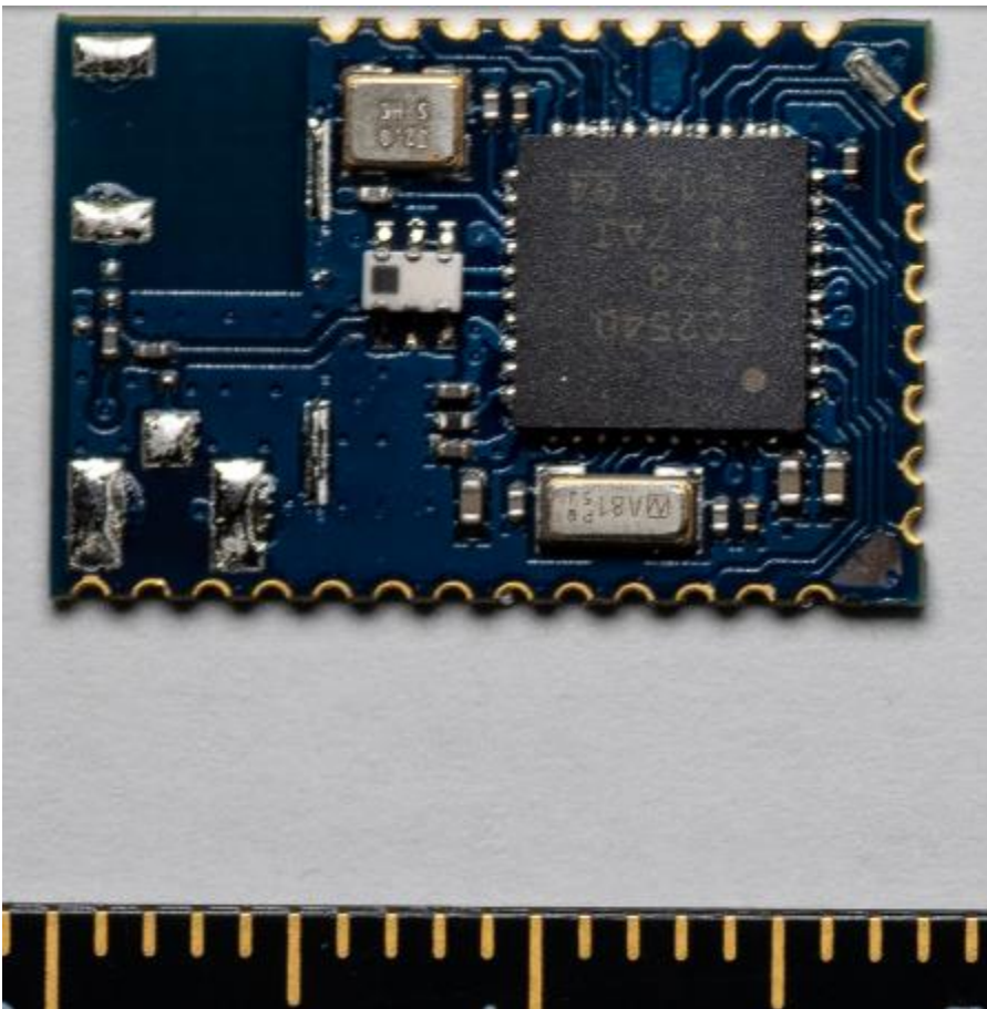
Figure 9 BLE112-N internal
