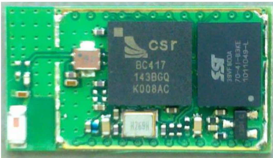
Figure 17 WT12-A internal
